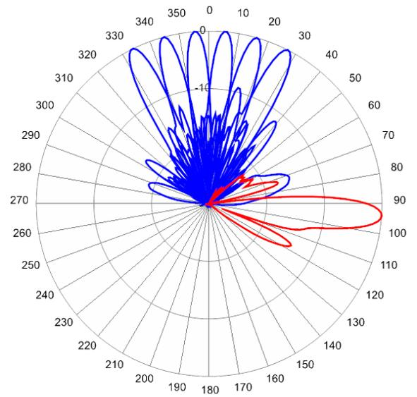
2650 MHz Azimuths with Elevation 4°
