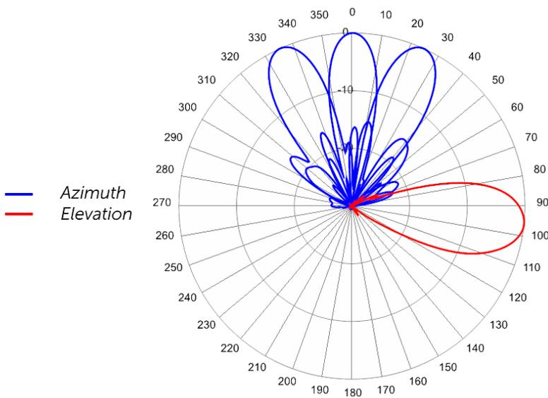
915 MHz Azimuth with Elevation 6°
